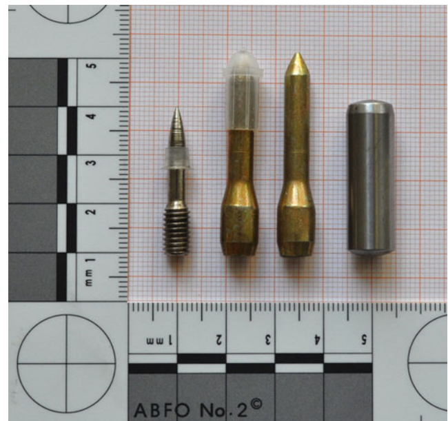
Fig. 2 Test projectiles. Left , 6-mm cal. threaded bolt (average mass, m=3.10 g; SD=0.13 g). Center , 8-mm cal. female-threaded steel dowels (average mass, m=6.40 g; SD=0.32 g) with and without plastic washer. Right , 10-mm cal. steel bolt (mass, m=18.68 g; SD=0.10 g)
